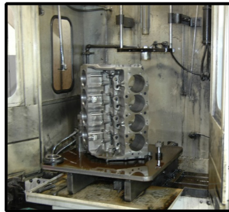
Block Prep Final lifter and hone spec. Finish machined to your specs. Final prepped and washed. Pipe plugs, cam bearings and freeze plugs installed. # BLOCK PRP
