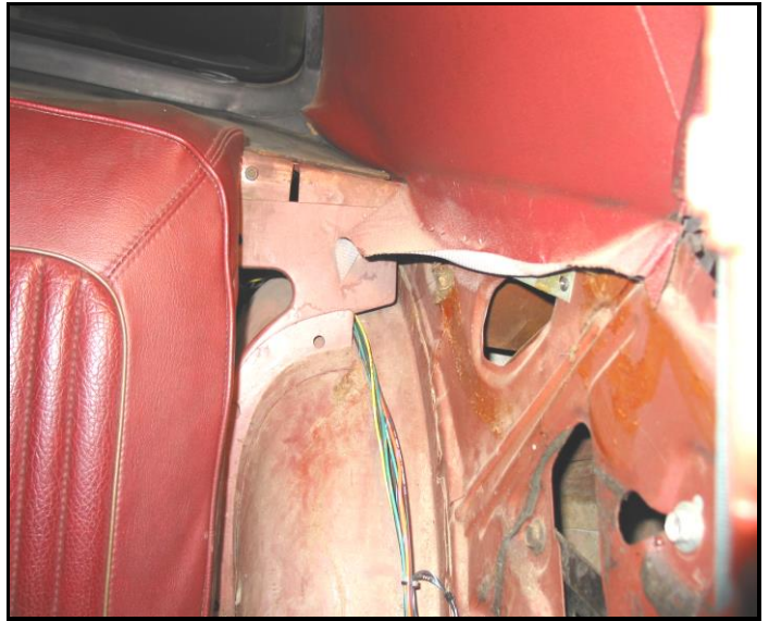
Figure 6-8D Tail Section Routing
