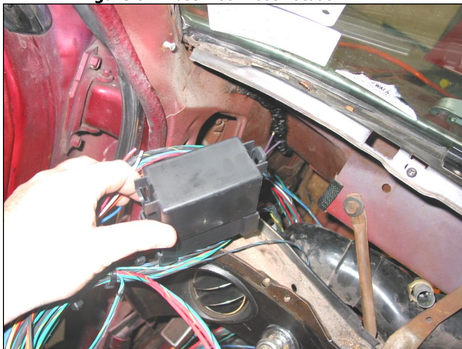
Figure 6-3 Routing Fuse Block through Instrument Cluster Opening
