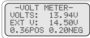
Press the (-Down) key and the POS and NEG cable results are displayed.
