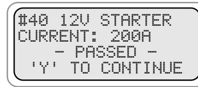
If the current is under 75A a solenoid connection or corrosion problem is likely and the following screens appear.
