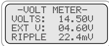
Note: If the car is running and the clamps are attached to the battery a high ripple (over 50.0 mv) indicates bad diodes in the alternator.
