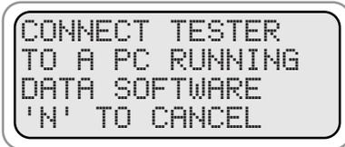
Using Auto Meter's optional adapter cord AC-12 insert the stereo plug into the jack on the BVA-350 and then plug the serial adapter into a free serial port on the rear of your computer or connect to AC-32 serial port to USB adapter. Follow the instructions of the AC-62 AMP Link Data Download software to retrieve data from the BVA-350.
