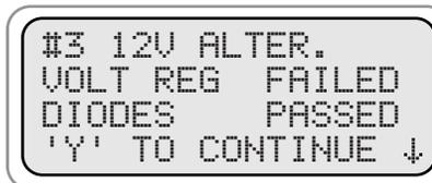
The alternator voltage regulator has failed and the voltage is either too high or too low.
