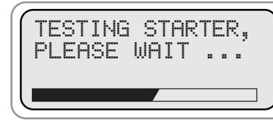
The BVA-350 will test the starting system. A bar at the bottom of the screen will show the tests progress.
