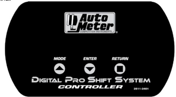
**B.) PLAYBACK MODE (Level 3 only)** – Press and release the **MODE (▲)** Button . The display will indicate “Play.” Press **ENTER(▼)** to confirm your choice and begin “playing back” the run stored in the memory on the display at 1/3 real time.
