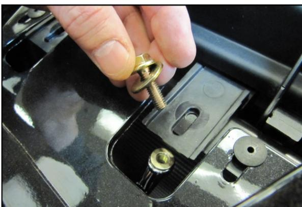
7. Using a 10mm box end wrench and socket, remove the two front airbox nuts and bolts in the core support.
