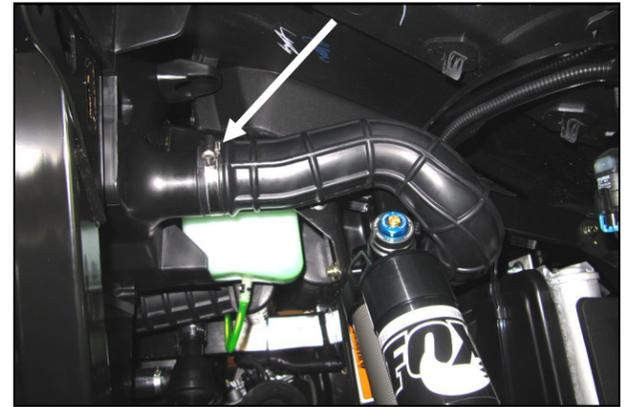
3. Loosen the firewall side clamp of the air inlet tube located in the passenger side front wheel well.
