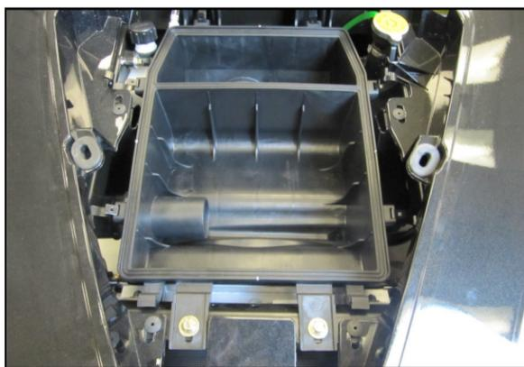
5. Remove the upper half of the airbox and the air filter.
