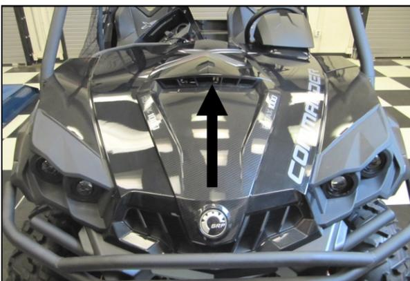
4. Remove the center section of the hood to gain access to the airbox assembly.
