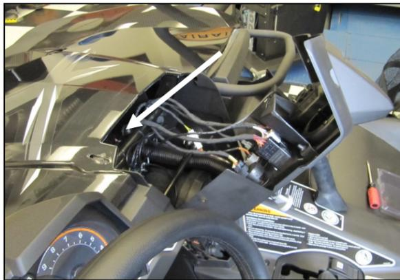
2. Pull the console back to gain access to the factory air intake. Loosen the throttlebody clamp.
