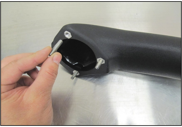
35. Install the Threaded Studs (#11) into the Riser Tube.
