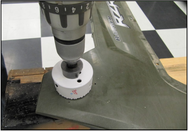
32. Cut the large hole in the panel using a drill with a 3" hole saw.
