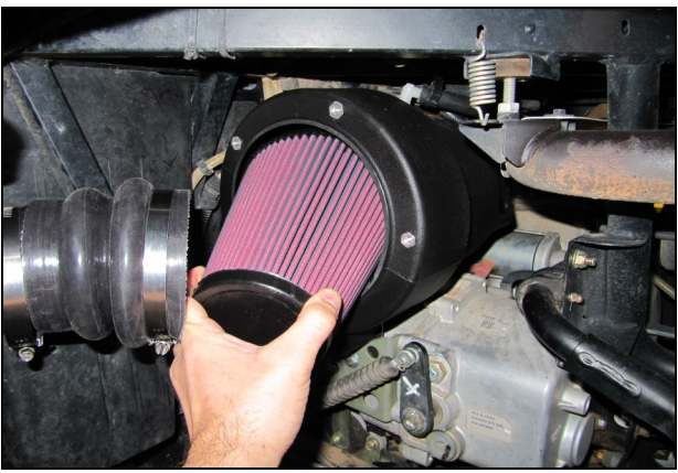
3. . The Filter can now be removed for service and inspection. Thoroughly inspect the interior of the Air Box for water and large pieces of debris that may have been ingested.
