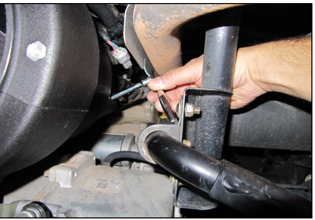
2. Remove the Plug Grommet in the access port and loosen the filter Clamp. A 1/4" drive ratchet with a 3" extension and a 5/16" socket works best.
