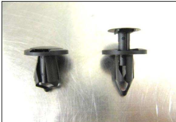
1. Many of the panels needing to be removed for this installation are held in place with the use of nylon rivets. Nylon rivets are reusable if care is taken during their removal and installation. Using a small standard blade screwdriver, gently pry up on the center post until the entire rivet can be pulled freely from the panel. Rivet installation is the opposite.
