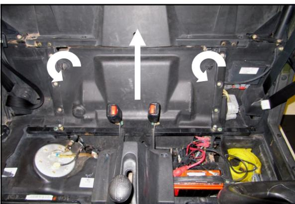
3. Remove the front engine cover by rotating the two twist locks counter clockwise and lifting out.
