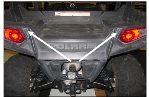
5. Using a T-25 Torx driver and a 7/16" wrench, remove the two outer bed bolts.
