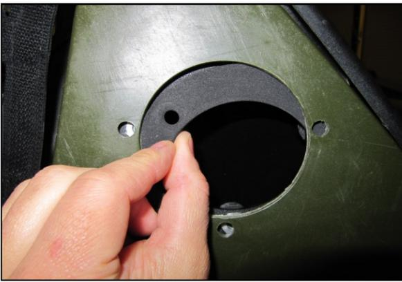
**43.** Place the Gasket between the Riser Tube and the Panel. Align the bolt holes.
