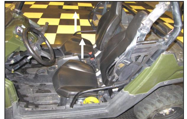
2 Place the range selector in Park. And remove both driver and passenger seats. Disconnect the negative terminal on the battery.
