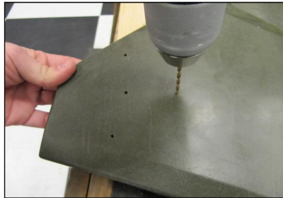
**31.** Drill four 1/8" pilot holes in the panel.
