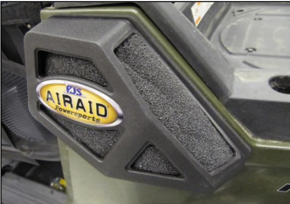
**3.** Insert the Foam Pre Filter (#6) into the Air Scoop as shown. Apply the Airaid Decal as shown.
