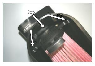
**5.** Locate the "step" on the bottom of the factory airbox. Make sure that the tab on the air filter is aligned with it. Next, align the two side tabs on the air filter with the side of the factory airbox.
