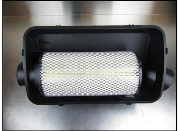
**1.** It is important to note that the Airaid RZR 1000 Air Filter is installed in the air box differently than the OEM filter.
