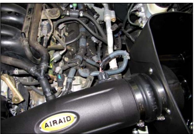
12. Reconnect the factory PCV breathers and spring clamps to the Barbed "Y" Fitting. Reconnect the Mass Air Flow sensor.
