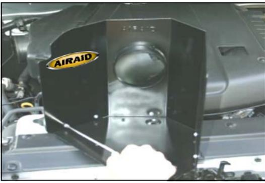
10. Assemble the Cool Air Dam panels (#2), and (#3) using the six supplied screws (#9), washers (#10), and nuts (#11.). Apply the Airaid Foil Decal onto the Panel as shown
