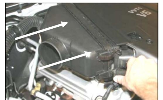
9. Re-install the factory airbox cover, and re-latch both clips.
