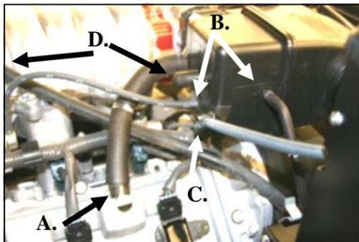
2. A) Disconnect the breather hose at the valve cover. B) Disconnect 1/4" and 1/8" vacuum lines on the back of the factory intake tube. C) Unclip MAF wire harness retainer from the intake tube. D) *Sequoias and 2000-02 Tundras only; remove 3/8" vacuum hose between factory intake tube and metal fitting on top of the intake manifold. (Hose Not Shown)*
