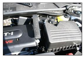
7. Reinstall the intake tube and air cleaner lid. Reconnect the mass air sensor wiring harness, and reinstall the harness holder into the air cleaner lid. Double check your work. Make sure all clamps, bolts, and connectors are tight.
