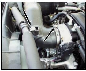
2. Loosen the hose clamp that holds the intake tube to the throttle body. Remove and save the bolt that holds the air conditioning line to the intake tube.
