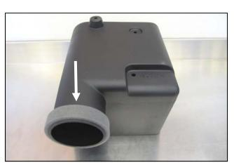
**6.** Apply the self adhesive, Foam Weatherstrip onto the air inlet on the Cold Air Box .
