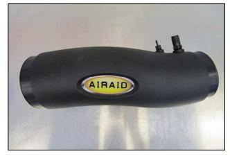
**9.** Install the 1/8" and 3/8" barbed fittings into the Airaid Intake Tube as shown. Apply the Airaid Decal onto the
