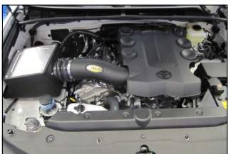
Make sure there is no foreign material in the and screws are tight. Double check the hood clearance!
