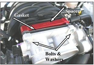
4. Install two bolts (#2), and washers (#3) thru the throttle body, thru the gasket (#4), thru the Poweraid Spacer (#1), and into the intake manifold as shown. Use caution to retain the factory o-ring gasket on the plastic intake manifold.
