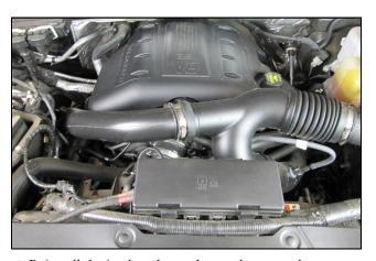
5. Reinstall the intake tube, and any other parts that were removed to gain access to the throttle body in the reverse order in which they were removed.
