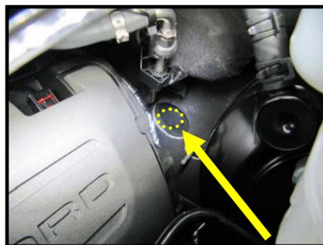
**Resonator Delete Option:** The resonator can be safely deleted if so desired by capping off the Intake Tube with the supplied Cap and Speed clamp. After removing the resonator assembly from the firewall, insert the included Firewall plug to prevent debris from entering the cabin.
