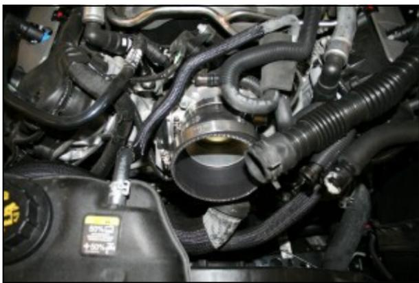
**10.** Install the Reducer and Hose clamps onto the throttle body. Place the #56 clamp on the Throttle body side of the reducer, and the #64 clamp on to the tube side.
