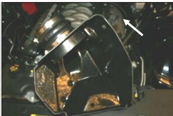
**8.** Install the hump hose onto the filter adapter using two #72 hose clamps as shown. Leave the two hose clamps loose for now. Transfer the Resonator stand off from the factory air box into the CAB.
