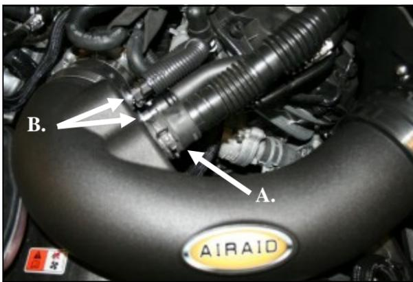
**11.** Install the Airaid Intake Tube into the couplers as shown, and tighten all Hose clamps. **A)** Reconnect the Resonator tube to the Airaid Intake using the OEM clamp. **B)** Reconnect the breather line/lines to the Aluminum Fittings depending on your application. Apply Airaid Decal As shown
