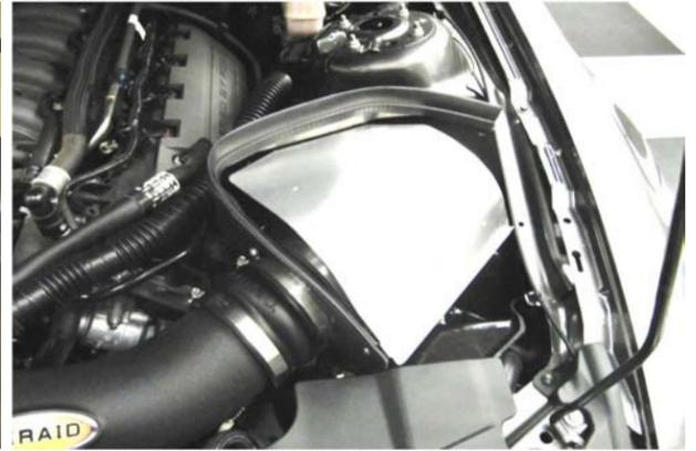
**15.** Install the Weather Strip onto the CAB with the contoured edge going away from the filter. Start at the front of the vehicle and work your way back. Replace the engine cover.
