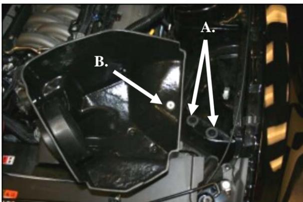
**7.** Transfer the factory air box mounting grommets. A) Locate and remove the Two Lower air box mounting grommets, and install them in the inner fender. B) Remove the Upper air box mounting grommet and steel sleeve, and re-install into the Airaid CAB.
