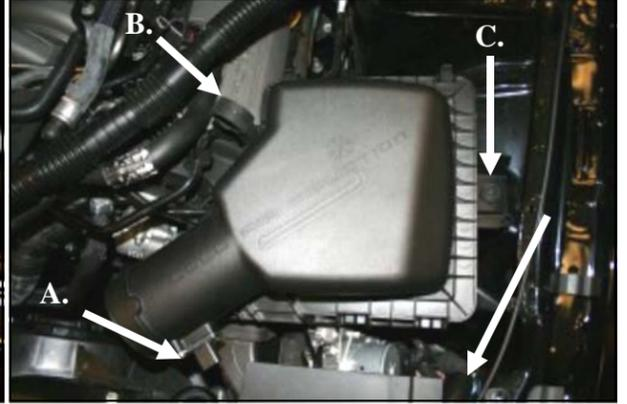
**3.** A) Slide the red tab, and disconnect the wiring harness from the Mass Air Flow sensor (MAF). Carefully pry the harness anchor from the air box using a screwdriver. B) Separate the resonator tube from the stand off attached to the Air box lid. C) Using a 10mm socket, remove the bolt securing the air box to the inner fender and remove the air box assembly. This bolt will be reused in
