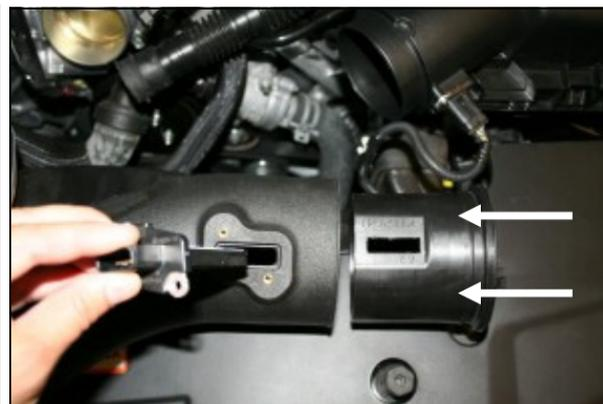
**5.** Using the supplied Torx driver, remove the MAF sensor from the Factory airbox and create the Tube assembly. A) Slide the Modular Venturi Tube into the Airaid intake tube making sure to align the two slots for the MAF sensor. B) Install the MAF sensor into the intake tube using two provided 8-32x3/8" screws. **Do Not Use The Factory Screws!**
