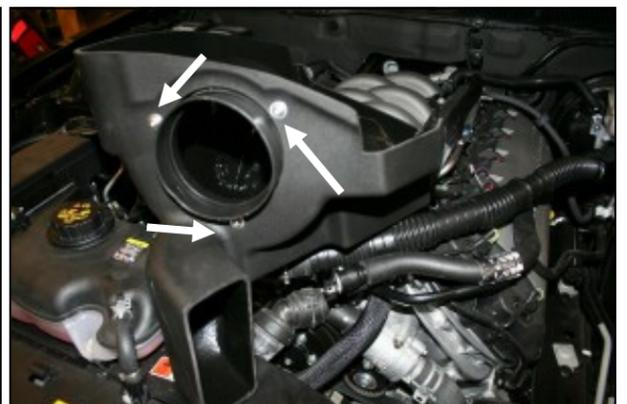
**6.** Install the filter adapter using three 1/4-20 button head bolts, and flat washers into the Airaid Cool Air Box (CAB) as shown.
