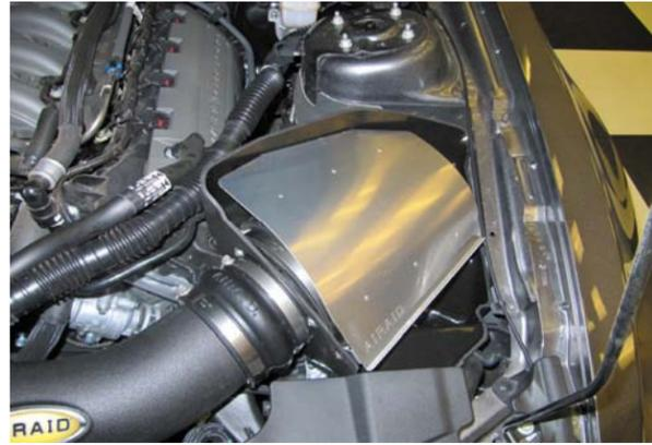
**14.** Mount the Rain Shield onto the Airbox as shown using the 1/4-20 Button Head Screws and Washers. **NOTE:** Installation of the Rain Shield is optional but highly recommended for vehicles with Power Dome hoods with heat extractors.
