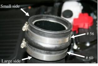
the **CAB** tube. Loosely install the #56 Hose Clamp (#10) on the small side of the Hump Hose, and the #60 Hose Clamp (#11) on the Large side. ( B) Slide the Hump Hose and Clamps downward on the tube, creating a compact assembly as shown.
