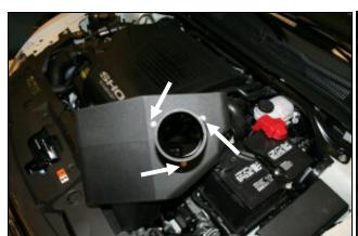
7. Install the Filter Adapter to the inside of the Cool Air 8. A) Install the Hump Hose, large side first (#4) onto 9. Remove the Air Temperature Sensor from the factory Box, CAB (#2) using the three 1/4"-20 hex head bolts (#6) and 1/4" flat washers (#7) as shown.
