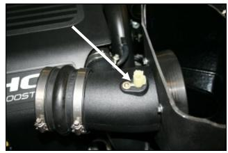
10. A) Transfer the factory Air Temperature Sensor into the Airaid Intake tube and align the sensor tab with the Groove in the tube. **B)** Secure the sensor to the tube using the 8-32 Button Head Bolt (#8) and the 3/4" washer
