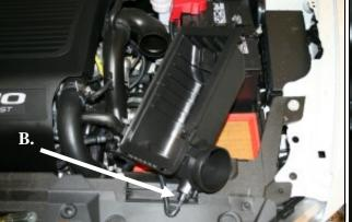
2.A.) Unfasten the factory air box clips and separate 3. Using a pair of needle nose pillars, carefully compress the upper half of the air box from the intake assembly. **B.**) Disconnect the air temperature sensor.
