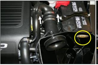
11. A.) Place the CAB in the original location of the 12.Install the Airaid Premium Filter (#1) onto the Filter Factory Air box and secure using the factory hardware adapter and tighten the clamp. from step 4. B.) Slide the coupler and clamps onto 90 deg. Elbow pipe and tighten the clamps. C.) Reconnect the Air Temperature Sensor. Apply the Airaid Decal inside of the Airbox as shown.
