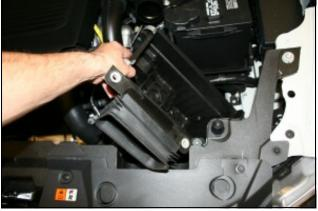
4. A.) Using an 8mm socket, remove the two factory 5. Remove the factory air box assembly from the vehicle. 6. Prepare the Filter Adapter (#3) for installation by posi-
