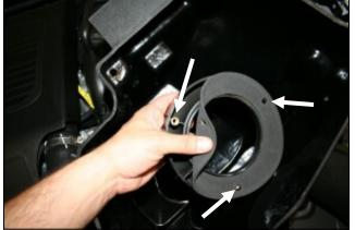
tioning the Adapter Gasket (#12) on the mounting side and lining up the holes.
