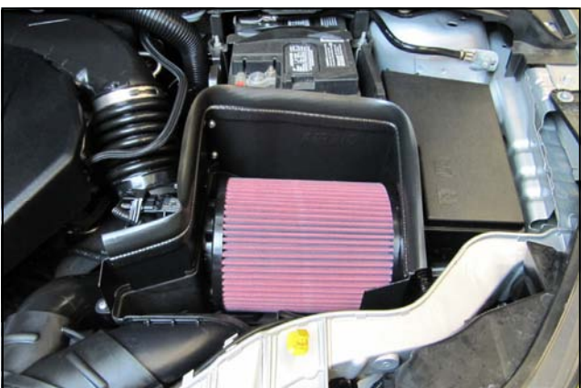
14. Install the Weather Strip (#4) onto the Panel assembly with the contour rolling away from the Air Filter.
