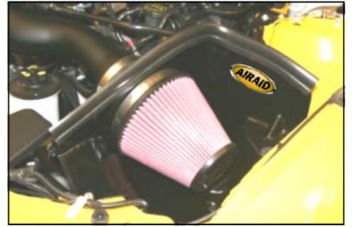
15. Install the Airaid Premium Filter (#1) onto the filter adapter (#5). Next install the weather strip (#7) on the top of the CAD as shown. Start at the front of the CAD and work towards the rear. Apply the Airaid Decal inside the CAB as shown.
