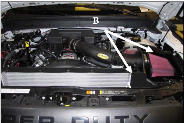
11. A) Install the Airaid Premium Filter (#1) to the mounting flange inside the quick fit assembly. B) Complete the installation by attaching the Weather Strip (#6) to the top of the panels as shown.
