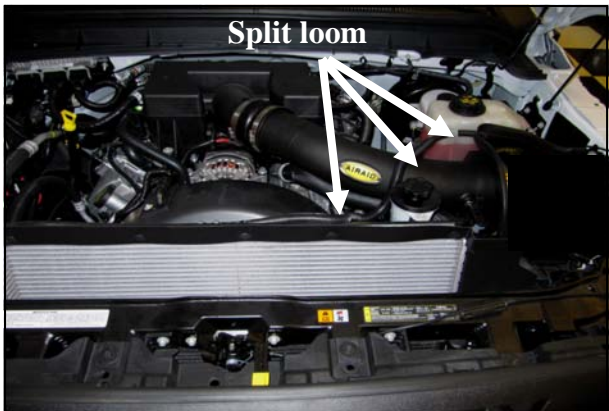
10. Slide the 20” section of Split Loom (#8) over the Coolant line to protect it from chaffing on the intake tube.
