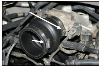
12. Install the small end of the reducing hump hose (#8) onto the throttlebody and tighten the #52 hose clamp (#20). Next, install the remaining #60 hose clamp (#21) on the large end of the hump hose leaving it loose for
