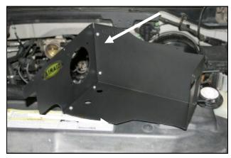
**6.** Assemble the MAF panel (#3), and bottom panel (#4) as shown using four 6-32 screws (#12), four flat washers (#13), and four Kep nuts (#14) as shown. Apply the Airaid Foil Decal onto the Panel as shown.
