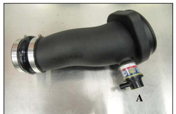
9. Create the Tube assembly. **A.)** Transfer the factory grommet and filter minder into the Airaid Intake Tube (#2). **B.)** Slide the Hump Hose (#10) and Clamps (#13) onto the Tube as shown. Leave the clamps loose for now.
