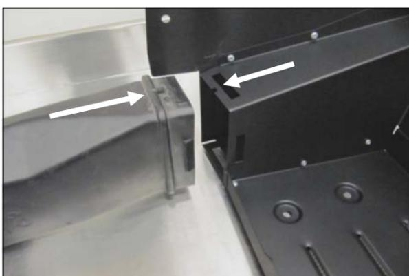
7. Transfer the air inlet from the factory airbox assembly into the CAD assembly. The air inlet has an indexing tab that mates with a slot in the Panel. NOTE: Vehicles built "BEFORE 12/7/98" do not have this air inlet design. This intake can be used with or without the factory inlet. It is available from Ford as a special order part. Ford Part number: 9C675 Engine Air Box Tube 7.3L "FROM 12/7/98"
