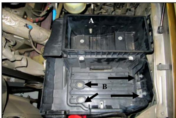
4. **A.)** Disconnect the air temp sensor.
