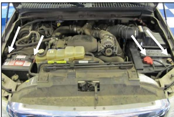
1. **Disconnect the battery cables.**
