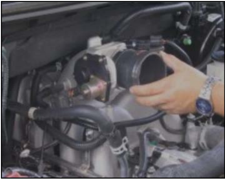
18. Install supplied silicone reducer on end of throttle body. Install #48 hose clamp on small end of the reducer and #56 hose clamp on the big end of the reducer. Leave hose clamps loose until final assembly.
