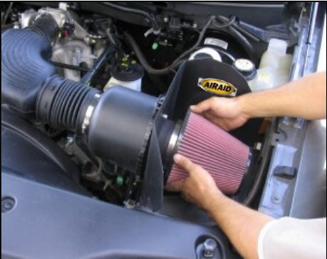
11. Mount the Airaid air filter on to the filter adapter using the supplied hose clamp.
