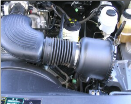
2. Remove air filter and air box from vehicle.
