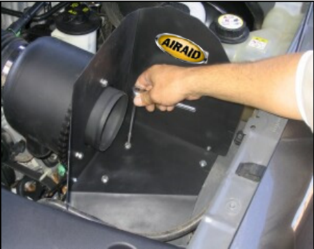
10. Finish mounting the Airaid Cool Air Dam assembly to body using the supplied ¼" nuts, bolts, washers and long bracket as shown. Note: The long bracket must be mounted under the factory mounting plate and grommets.
