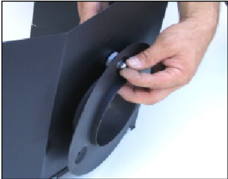
4. Assemble the Airaid Filter Adapter plate using the supplied ¼ inch bolts, washers, spacers and nuts provided as shown above.
