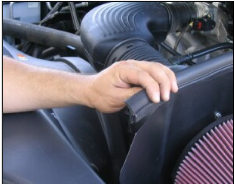
12. Install the supplied weather strip on the top edge of the Airaid Cool Air Dam. Note: The weather strip is pre cut to the proper length. Start from one end and work your way around to the other end to insure even placement.
