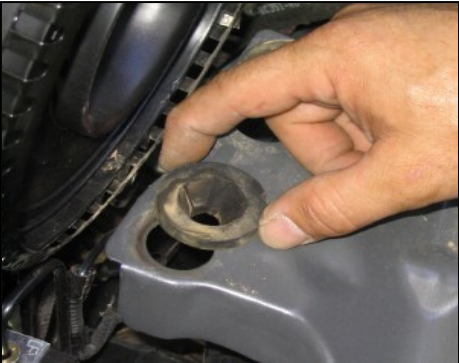
6. Remove the two factory grommets from the body and discard.
