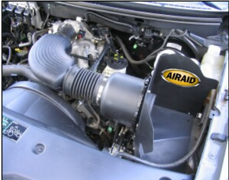
8. Install the Airaid Cool Air Dam assembly on vehicle using the factory intake tube clamp. Apply the Airaid Foil Decal onto the Panel as shown.
