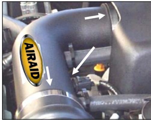
**11.** Install the 7/16" rubber grommet (#15) into the Airaid Intake Tube (#2). Insert the factory AIT sensor into the grommet. Slip the Airaid Intake Tube into the urethane hump and reducer hoses. Align for best fit and tighten the remaining hose clamps. Tighten the MAF bracket and reconnect the AIT sensor wiring harness. Apply the Airaid Bubble Decal onto the Intake Tube as shown.
