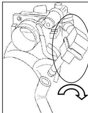
**14. 4.6L engines:** Rotate the IABV inlet tube 90 degrees to provide clearance for the 3/4 x 12" L-hose (#7).
