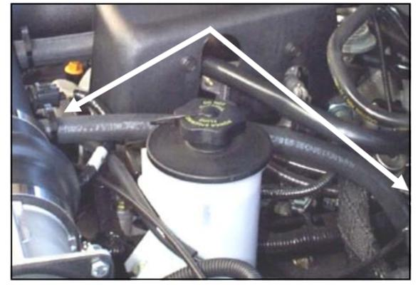
**12.** Install the 5/8"X18" breather hose (#6) onto the valve cover breather fitting then onto the Airaid Intake Tube nipple. Secure the hose using two #19 speed clamps (#16).
