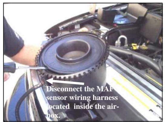
**6.** Locate the notch on the flat side of the airbox and gently pry it up. Disconnect the MAF sensor wiring harness from the sensor (inside the air-box).
