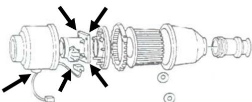
**7.** Using a 10mm socket, remove the four MAF sensor mounting nuts. Carefully remove the MAF sensor and the wiring harness from the airbox, (save them for reuse).
