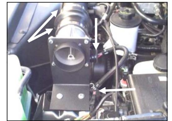
**9.** Reconnect the MAF sensor wiring harness to the sensor, and to the main engine wiring harness. Install the urethane hump hose (#4) onto the MAF sensor, with two #60 hose clamps (#13). Tighten only the clamp on the sensor.
