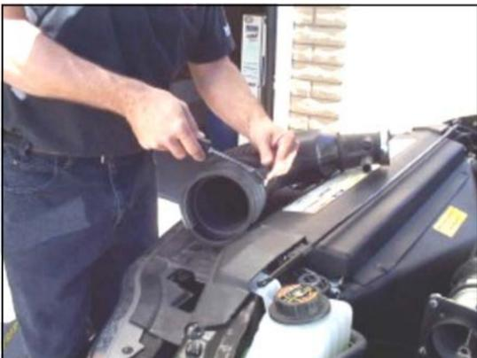
**4.)** Remove the factory intake tube, and set it aside. Remove the AIT sensor from the tube by carefully prying it out with a flat blade screwdriver (save the sensor for reuse). Disconnect the Mass Air Flow (MAF) sensor wiring harness from the main engine wiring harness.
