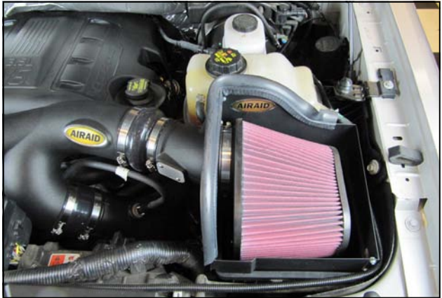
15. Install the Airaid Premium Filter onto the Sensor Tube and tighten the clamp.
