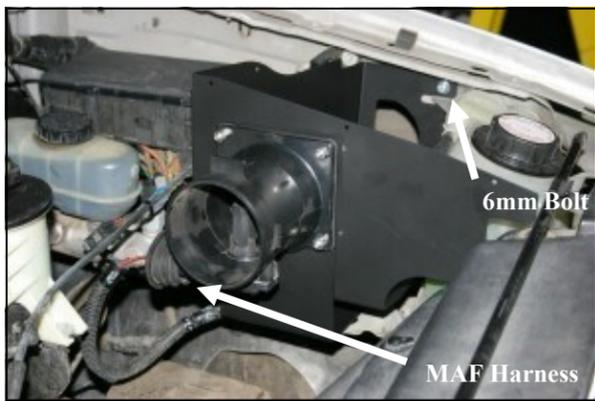
**10.** Install the CAD assembly into the vehicle using two 1/4-20x7/8" bolts (#15), four 1/4" flat washers (#16), one MAF backing plate (#19), and two 1/4" nylock nuts (#17). Leave the two bolts slightly loose for now for final adjustment. Refer to the line drawing on page 1 for reference. Next, reinstall the 6mm bolt through the CAD, radiator overflow tank, and into the fender well. Reconnect the MAF sensor wiring harness.
