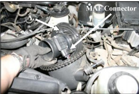
4. Unlatch the clamp on the canister to separate the two halves. Once separated, remove the factory air filter. **A)** Next, slide the large round plastic Mass Air Flow (MAF) sensor adapter plate from the canister. To do this, slide the wires through the rubber grommet to gain access to the MAF sensor wiring connector. Now disconnect the MAF sensor wiring harness, and remove the MAF sensor housing and adapter plate. Remove the remaining half of the canister from the vehicle.
