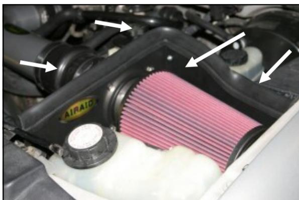
**16.** Reinstall the beauty cover using the 3 factory bolts. Install the Airaid Premium Filter (#1) as shown, and tighten the hose clamp.
