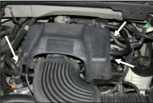
1. **Disconnect the negative battery cable.** Using a 10mm socket, remove the three bolts that secure the beauty cover over the throttlebody. Remove the cover and save these parts for reinstallation in step #16.
