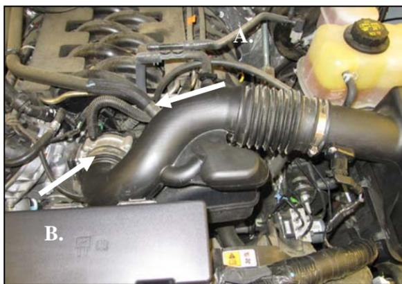
2. A. Disconnect the two breather lines in the factory intake tube .
