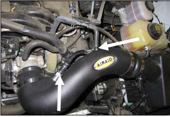
10. Reconnect the breather lines to the Airaid Intake Tube.
