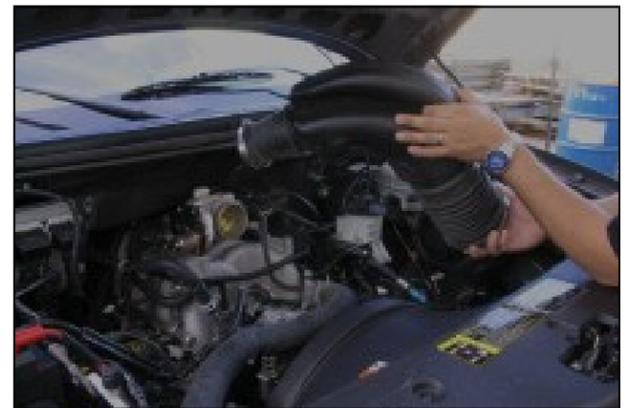
**3.** Remove the factory intake tube assembly from engine.
