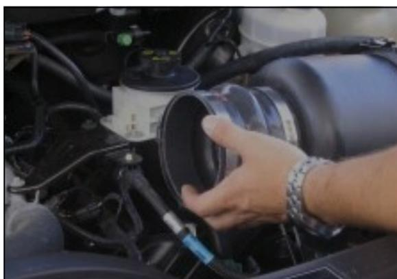
**5.** Install the supplied urethane hump hose and two #80 hose clamps on factory air filter assembly. Leave hose clamps loose until final assembly.
