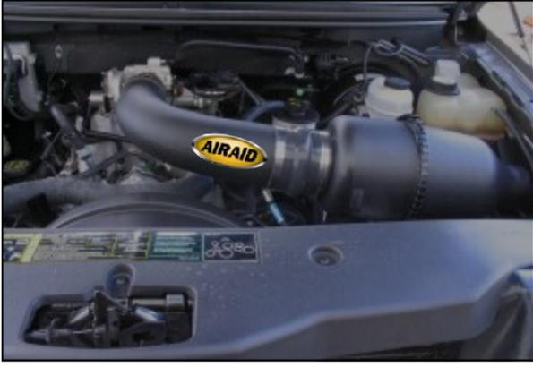
10. Double check your work to be certain that all nuts, bolts, and clamps are securely fastened. Apply the Airaid Bubble Decal onto the Intake Tube as shown.
