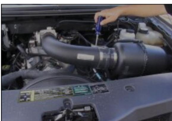
**8.** Tighten hose clamps on both ends of the Modular Intake Tube.
