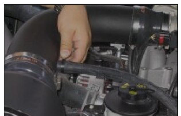
**9.** Install the supplied rubber hose on the Modular Intake Tube. Connect the other end of the hose to the valve cover. Secure both ends of the hose with the supplied speed clamps.
