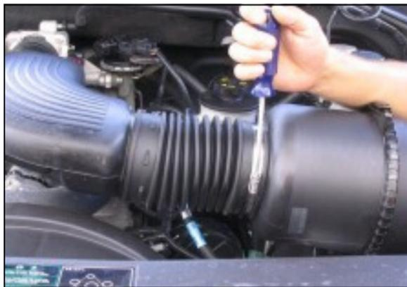
**2.** Loosen hose clamps connecting the factory intake tube to the air filter assembly and throttle body.
