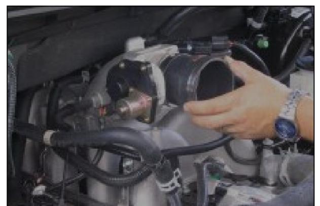
**6.** Install supplied silicone reducer on end of throttle body. Install #48 hose clamp on small end of the reducer and #56 hose clamp on the big end of the reducer. Leave hose clamps loose until final assembly.
