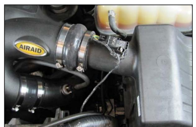
**9.** Reconnect the air meter or Map sensor and tighten all Clamps.
