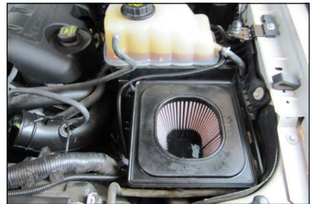
**3.** If installing an Airaid Jr. kit, replace the factory air filter with the Airaid Premium Filter at this time.
