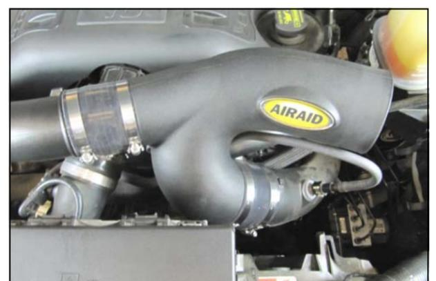
**6.** Install the Airaid Intake Tube onto the factory turbo plumbing and tighten the Clamps. Reconnect the vacuum line if so equipped
