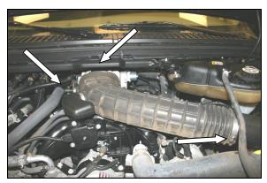
1. <u>Disconnect the negative battery cable!</u> Push the green locking tab on the factory breather hose, and disconnect it from the intake tube. Loosen the two hose clamps at each end of the factory intake tube. Remove the tube from the throttle body, and the factory air cleaner, and set it aside.
