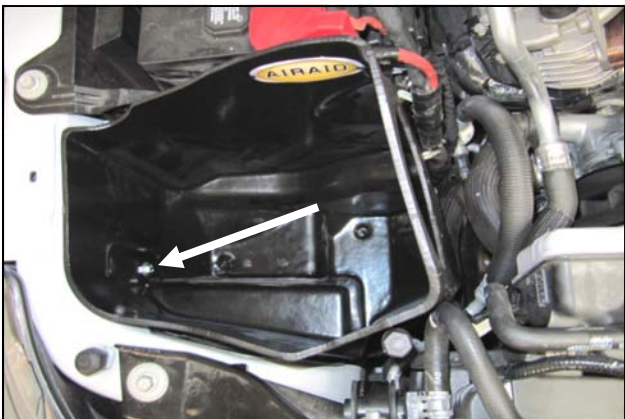
11. Place the CAB into the engine compartment and secure to the inner fender using the M8 x 1.25 x 30 hex Head Bolt (#10) and the 8mm Flat washer (#12). Apply the Airaid decal to the CAB as shown.
