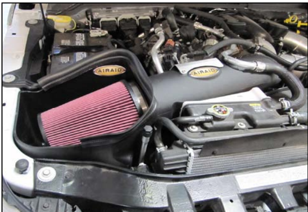
18. Install the Airaid Premium Filter (#1) inside the CAB and complete the install by trimming the CAB with the Weather Strip (#6).
