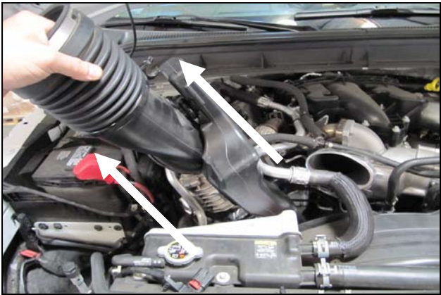
7. Unclip the coolant hoses from the intake tube and resonator, and remove it from the vehicle.
