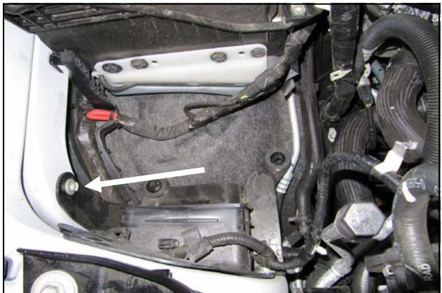
5. Using a 13mm socket, remove the 8mm inner fender bolt.
