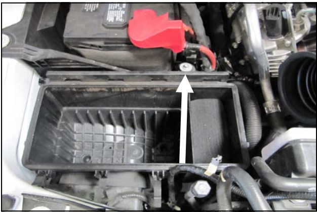
4. Using a 10mm socket, remove the 6mm bolt securing the lower half of the airbox to the vehicle. Remove the airbox from the vehicle.
