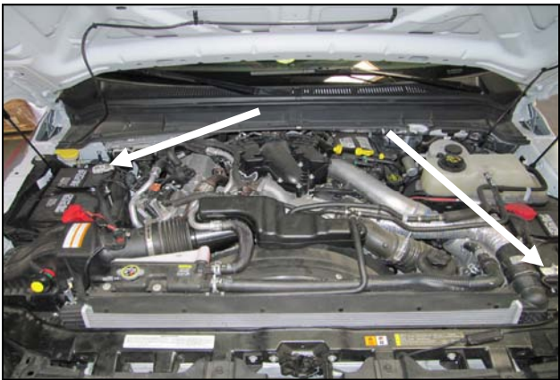
1. Disconnect both of the negative battery cables.
