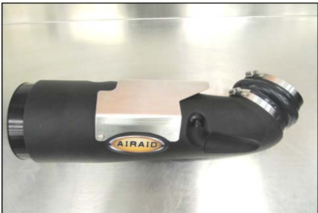
12. Slide the Hump Hose (#5) and Clamps (#14) onto the Airaid Intake Tube. Leave the clamps loose for now.
