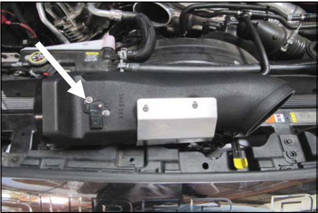
9. Transfer the Mass Air Flow sensor, or M.A.F., from the factory airbox lid into the Airaid Intake Tube and secure using the supplied 8-32 x 1/2 Button Head Bolts (#8). Do Not Use The Factory Hardware.
