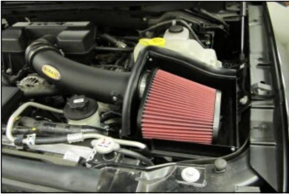
**10.** Install the Airaid Premium Filter (#1) to the mounting flange inside the quick fit assembly.
