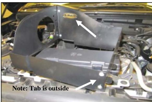
**4.** Assemble the two Quick Fit panels (#3 & #4) as shown using four 6-32 screws (#7) flat washers (#9) and keps nuts (#8). Apply the Airaid Foil Decal to the Panel assembly as shown.
