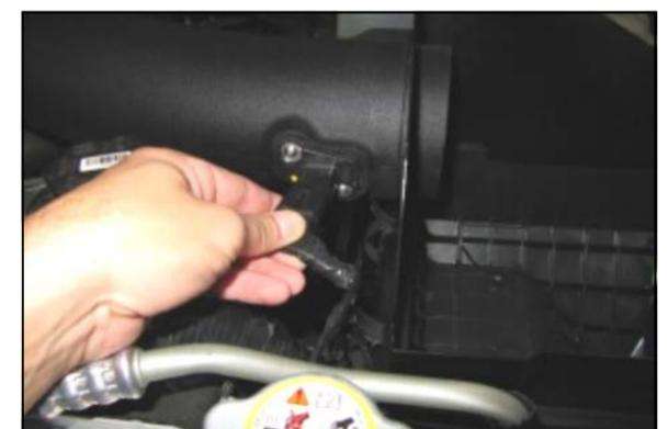
**9.** Re connect the Mass Air Flow Sensor.
