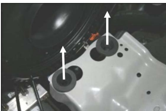
**7.** Remove the two factory grommets from the factory airbox mounting plate.
