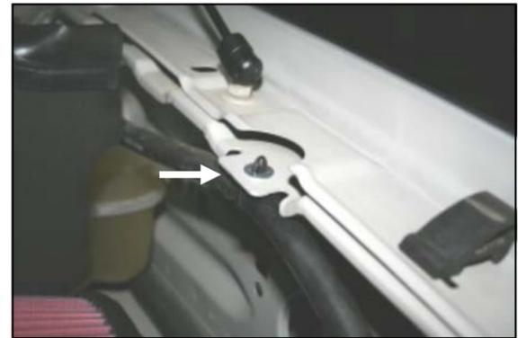
**15.** Slip the black plastic hose mount (#17) over the radiator overflow hose. Next, place one 1/4" flat washer (#10) over the hole on the inner drivers side fender. Slide the hose mount prongs thru the fender and thru the washer.
