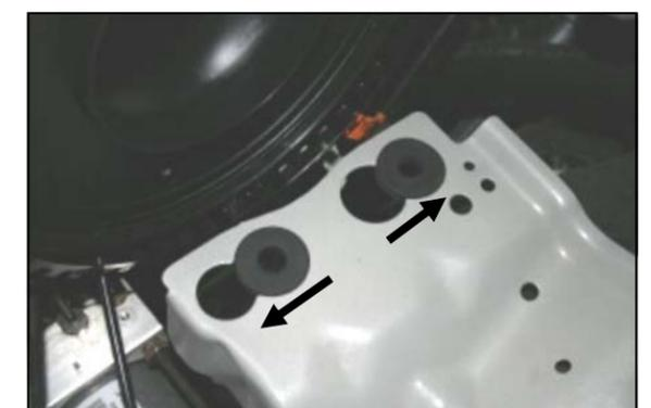
**9.** Slip two rubber grommets (#14) into the large holes in the factory airbox mounting plate, and then slide them sideways into the small holes as shown.
