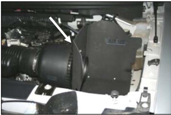
**10.** Install the CAD assembly into the vehicle. First, align the filter adapter with the factory MAF sensor housing, then, secure it with the factory clamp.
