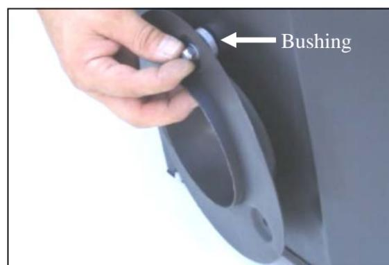
**5.** Insert three 1/4-20 x 7/8" bolts (#9), and 1/4" flat washers (#10) through the CAD. Place one bushing (#11) at each hole between the CAD and the filter adapter (#4). Next, secure the assembly using three 1/4" flat washers (#10), and 1/4-20 nuts (#12).
