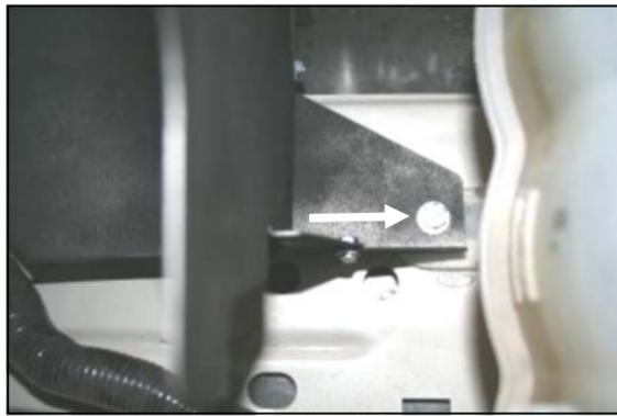
**11.** Align the hole in the CAD with the hole in the factory coolant reservoir mount. Insert one M6-1x25 hex bolt (#15) and 1/4" flat washer (#10) through the hole in the CAD, through the coolant reservoir mount, and into the speed nut below it.
