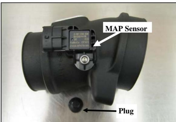
**8.** Transfer the MAP Sensor into the Airaid Sensor Tube as shown. Secure the sensor using the Long 8-32 Button Head Screw and the Washer. Discard the Plug. It will not be used.
