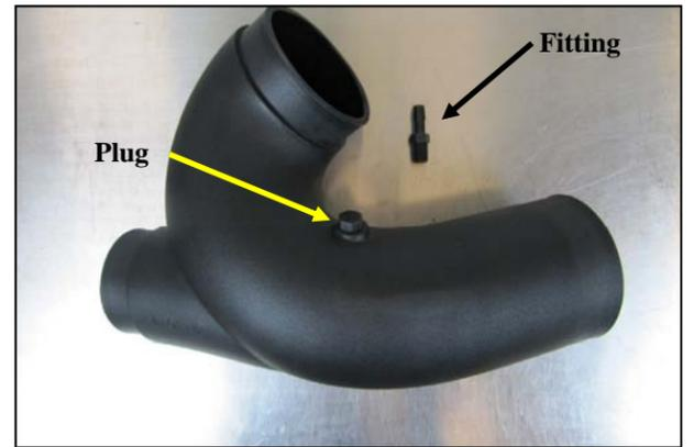
**3.** On 2011 models with the vacuum line in the intake, install the 1/4" Barbed Fitting. The Plug will not be used. On 2012-2014, Install the 1/4" Plug into the Airaid Intake Tube as shown.
