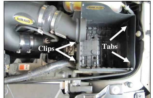
**12.** Install the Tube and Panel assembly onto the Airaid Intake Tube first, then insert the Panel tabs into the factory air box slots. Adjust the assembly until the OEM air box clips can positively engage the Panels and lock.
