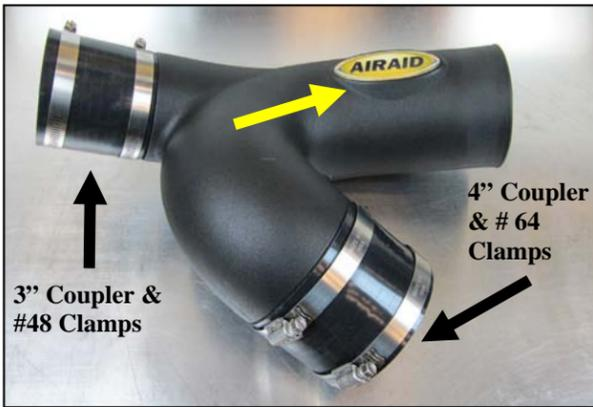
**4.** Slide the Couplers and Clamps onto the Intake tube as shown. Complete the Tube assembly by applying the Airaid Bubble decal.
