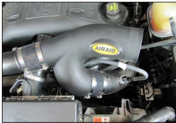
**5.** Install the Airaid Intake Tube onto the factory turbo plumbing and tighten the Clamps. On 2011 models, reconnect the vacuum from step 1 to the Fitting installed in step 3.
