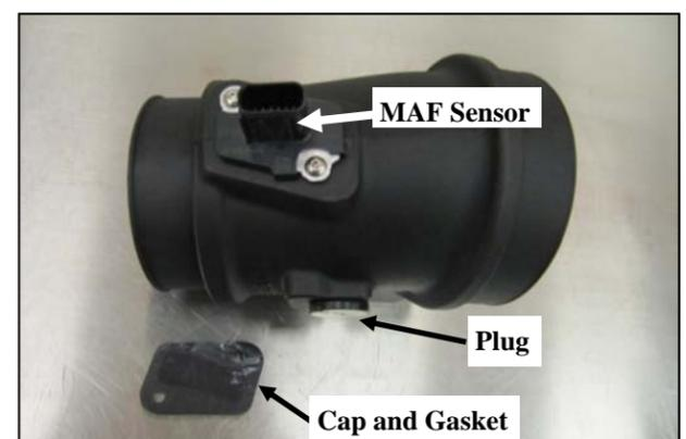
**9. If your vehicles intake utilizes a Mass Airflow, or MAF sensor:** Transfer the sensor into the Airaid Sensor Tube as shown and secure using the two 1/2" Button Head Screws. Complete the Tube assembly by inserting the MAP Plug. Discard the Meter Cap and Gasket. They will not be used.
