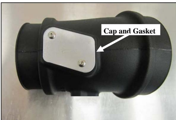
**7. If your vehicles intake utilizes a MAP sensor:** Install the Meter Cap and Gasket onto the Airaid Sensor Tube as shown, using the two 8-32 1/2" Button Head Screws.
