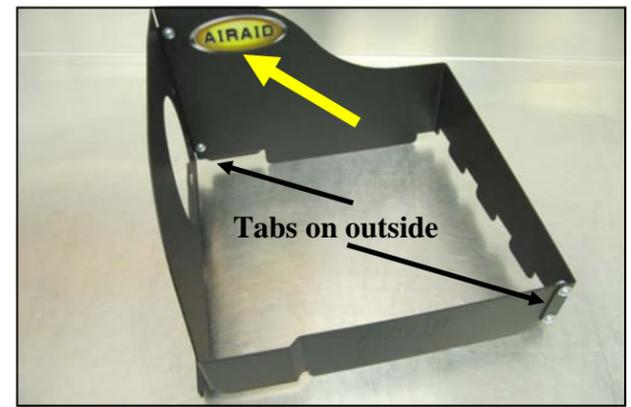
**6.** Assemble the Front and Rear Panels as shown with the tabs on the outside of the assembly. Use the four 6-32 Phillips Head Screws, #6 Flat Washers, and #6 Kev Nuts to secure the assembly. Complete the Panel assembly by applying the Airaid Foil decal.
