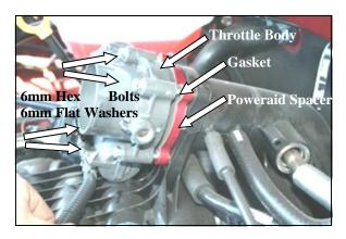
**4.** Install the Poweraid Spacer (#1) with the bore extending into the intake manifold. Install the Gasket (#2) between the Poweraid Spacer and the throttle body. Install four 6mm x 50mm hex bolts (#3) and 6mm flat washers (#4) through the throttle body, Poweraid Spacer, Gasket, and into the intake manifold. Using a 10mm socket, tighten all four throttle body bolts evenly, to the manufacturer's specifications. **Do Not Over Tighten The Bolts!** Reference picture below for spacer orientation.
