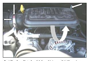
**2. All other listed vehicles:** Using a 5/16" socket, or flat blade screwdriver, loosen the hose clamp which secures the factory intake tube to the resonator box. Disconnect the factory temperature sensor wiring harness from the sensor in the resonator box. Slide the factory intake tube off of the resonator box. Remove the resonator box by pulling straight forward to release it from the throttle body and the grommet mounts. Save the resonator box for reuse.
