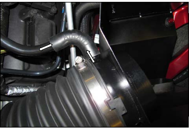
15. On V6 motors, connect the factory crankcase breather hard line to the Airaid Intake Tube using the 90 deg. Breather Elbow (#7). Disregard the 13" Breather Hose (#6) it will not be used.
