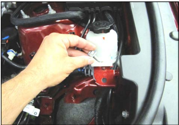
12. Remove the bolt securing the power steering reservoir and set it aside. This bolt will be reused in step 13. to hold the Mounting bracket.
