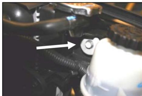
8. With a 10mm socket, remove and save the bolt that holds the radiator to the radiator support. It will be reused in step #10.
