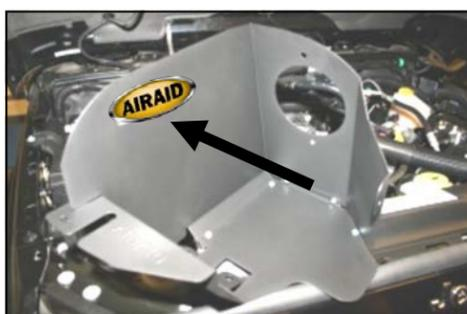
11. Assemble the Cool Air Dam panels (#3 & 4) as shown, using the seven 6-32 screws (#10), flat washers (#11), and keps nuts (#12). Apply the Airaid Decal as shown.
