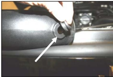
14. Install the supplied grommet (#17) into the Airaid Intake Tube (#2).
