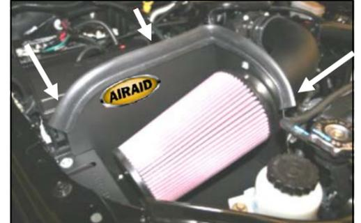
18. Install the Airaid Premium Filter (#1) onto the intake tube, and tighten the clamp. Next install the weatherstrip (#6) onto the top of the CAD as shown.
