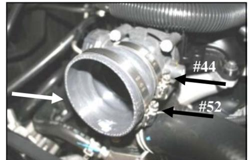
15. Install the reducing hump hose (#5) onto the throttle body as shown, with the #44 hose clamp (#15) on the back, and the #52 hose clamp (#16) on the front. Leave the clamps loose for now.
