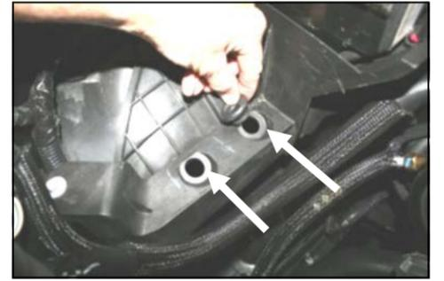
6. Remove the 2 lower grommets from the factory plastic air cleaner mount.
