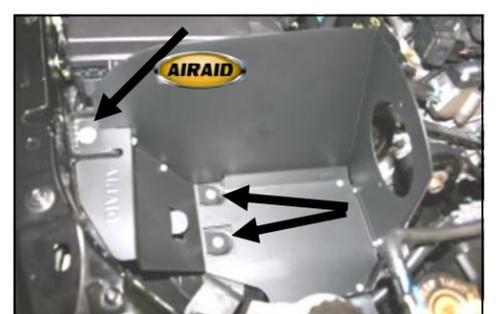
12. Install the CAD into the vehicle. Install the two 3/8 x 1 1/4" button head bolts (#13), thru the bottom panel, and into the well nuts. Reinstall the factory bolt removed in step #7 thru the panel, and into the fender well. Tighten all three bolts at this time.
