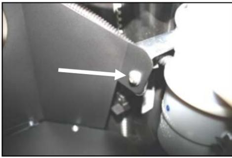
13. Using one 1/4" button head bolt (#7), 1/4" flat washer (#8), and 1/4" serrated nut (#9), attach the CAD panel to the L-bracket, as shown. Now tighten the radiator mounting bolt on the other end of the L-bracket.
