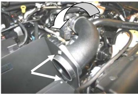
16. Install the Airaid Intake Tube into the hump hose first, and then rotate it down, and into the CAD. Install two 1/4" button head bolts (#7), and 1/4" flat washers (#8) thru the CAD, and into the inserts in the tube. Adjust for fit, and tighten both hose clamps, and bolts.
