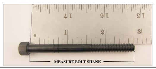
3. Measure your OEM hardware to determine which Poweraid bolts you will need. Measure the shank only. Use the chart below to select the proper bolts.
