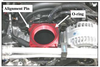
**4.** Install the supplied o-ring into the groove on the Poweraid Spacer. Next install the spacer onto the intake manifold with the o-ring facing up, making sure that the alignment pin holes are located over the alignment pins.
