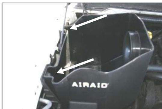
**8.** Install the CAB into the vehicle by aligning the grommets over the locating pins on the factory airbox mount. Reinstall the factory bolts thru the CAB and into the fender that were removed in step #4.
