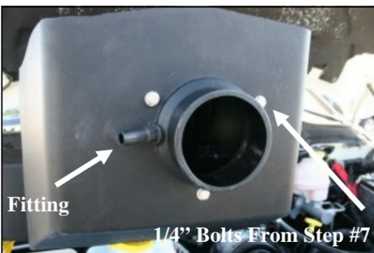
**7.** Install the 1/4" NPT x 1/2" barbed fitting (#8) into the filter adapter as shown.
