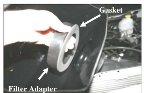
**6.** Install the adapter gasket (#12) and filter adapter (#3) into the CAB using three 1/4-20 x 5/8" bolts (#5) and flat washers (#6) as shown. Refer to the line drawing above for reference.
