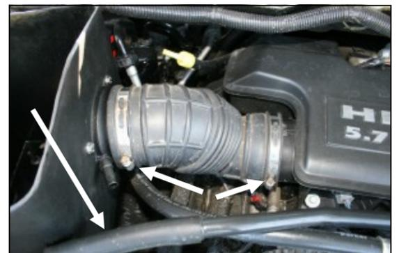
**9.** Reinstall the factory air intake tube and tighten the two hose clamps. Remove the rubber hose from the end of the factory crankcase breather tube.
