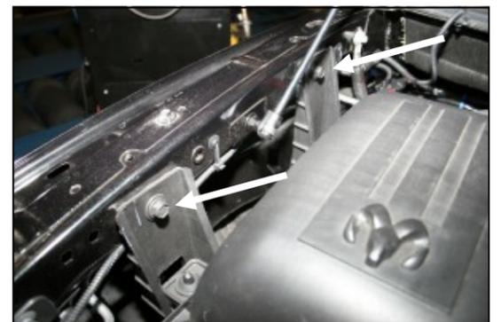
**3.** Using a 13mm socket, remove the two bolts that hold the air cleaner mount to the inside right fender. Save them for reinstallation in step #9.
