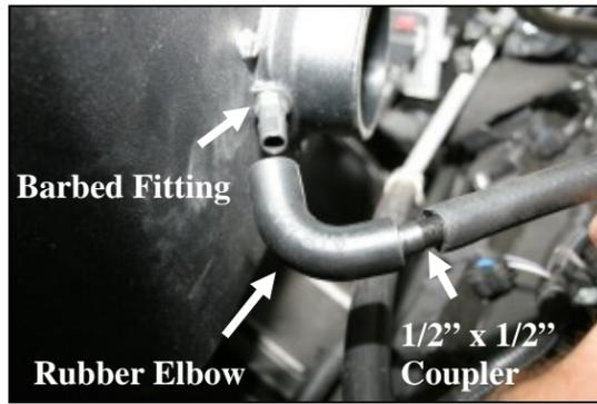
**11.** Install the supplied 1/2" x 1/2" plastic coupler (#11) into the 1/2" hose from step #10. Next connect the 1/2" rubber elbow (#8) between the 1/2" connector and the barbed fitting on the filter adapter.
