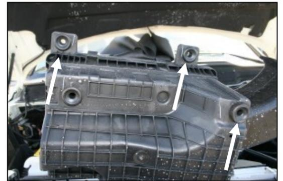
**3.** Remove and save three grommets from the bottom of the factory airbox. They will be reused in step #4.
