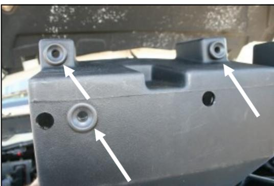
**4.** Install the three grommets removed in step # 3 into the bottom of the Airaid Cool Air Box (CAB) (#2) at the locations shown here.
