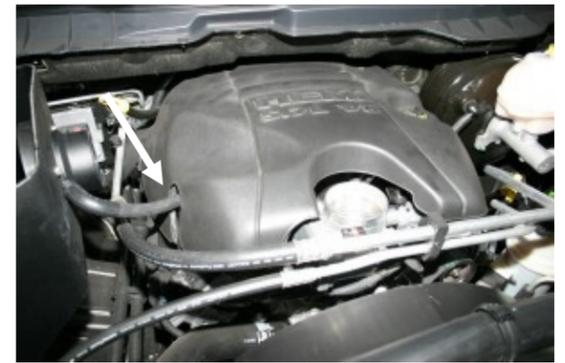
**12.** Reinstall the factory beauty cover making sure that the grommets are aligned with the grommet posts and that the crankcase breather hose is aligned in the slot on the side of the cover.
