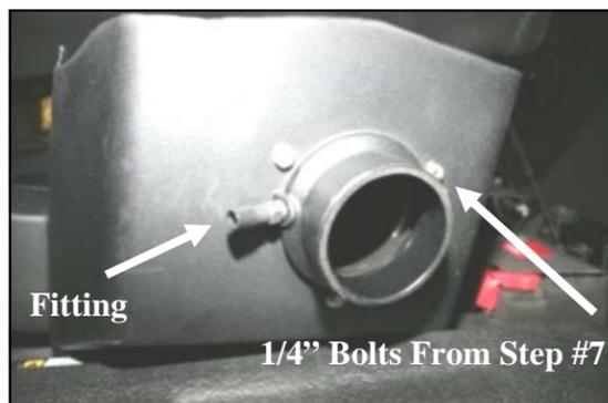
**8.** Install the 1/4" NPT x 1/2" barbed fitting (#9) into the filter adapter as shown.
