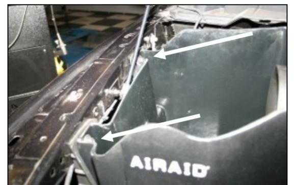
**9.** Install the CAB into the vehicle by aligning the grommets over the locating pins on the factory airbox mount. Reinstall the factory bolts into the fender that were removed in step #3.
