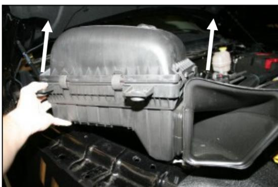
**4.** Rock the airbox back and forth as you are lifting it straight up to remove it from the vehicle. It is only held in by grommets.
