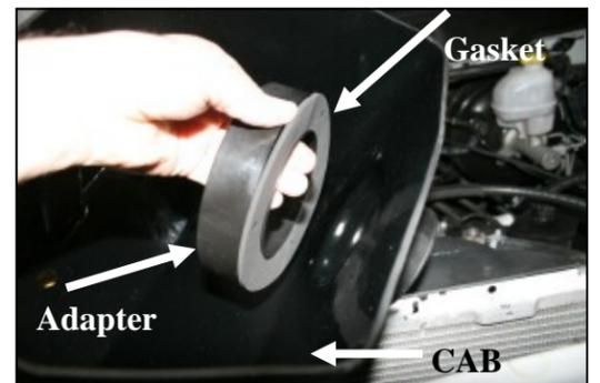
**6.** Install the filter gasket (#23) and filter adapter (#6) onto the Airaid Cool Air Box, or CAB (#3) as shown using three 1/4" x 5/8" bolts (#8), and 1/4" flat washers (#9). Refer to the line drawing above for reference.
