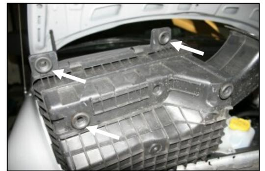
**3.** Turn the factory air box over and remove 3 of the 4 grommets. They will be reinstalled in the Airaid Cool Air Box in step #8.
