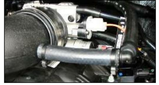
15. 2002-03 Models: Install one end of the provided 90° barbed fitting (#22) into the factory breather hose and then connect the supplied 1/2" breather hose (#21) to the other end. Connect the hose to the nipple on the Airaid intake tube. Secure all three connections with the provided #16 Speed Clamps (#17).
