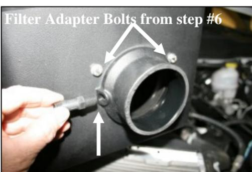
**7. 2004-12 Models:** Install the 1/4" NPT x 1/2" Barbed fitting (#18) into the CAB as shown. **2002-03 Models** Install the 1/4" hex plug (#19) in place of the barbed fitting.
