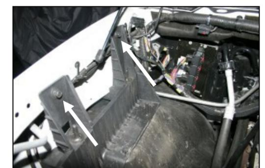
**9.** Remove the two bolts that secure the factory airbox mounting bracket to the inner fender. They will be reinstalled in step #10.
