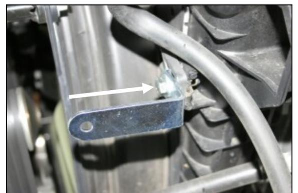
**6.** Install the L-bracket (#20) onto the radiator shroud as shown using one M8 x 30mm bolt (#14) and one flat washer (#12) as shown. Leave the bolt slightly loose for now.
