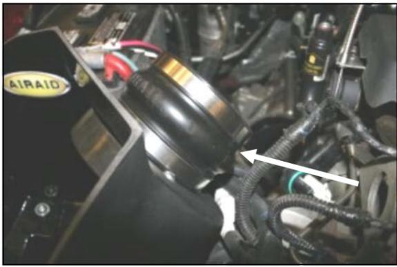
**10.** Install the supplied hump hose (#5) onto the filter adapter using two #72 hose clamps (#19). Leave the clamps loose for now. Apply the Airaid Bubble Decal inside the Airbox as shown.
