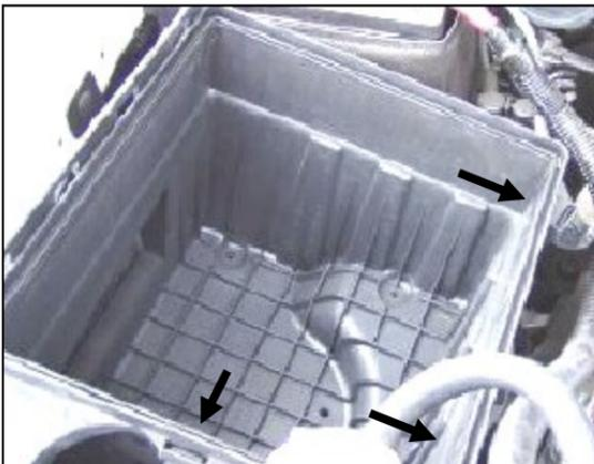
**4.** Unlatch the three clips on the factory air box. Remove the factory intake tube assembly and air-box lid from the vehicle.
