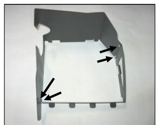
**9.** Assemble the Airaid Cool Air Dam (CAD) panels (#2,#3) using four 6-32x 5/16" screws (#7), #6 flat washers (#8) and 6/32 keps nuts (#9).
