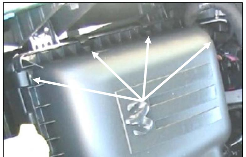
**2.** Unlatch the four factory airbox clips, and then remove the airbox lid and air filter from the factory airbox base.
