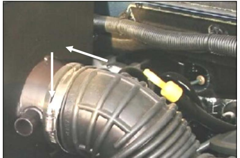
**4.** Reconnect the factory intake tube onto the CAD, and tighten the factory hose clamp.
