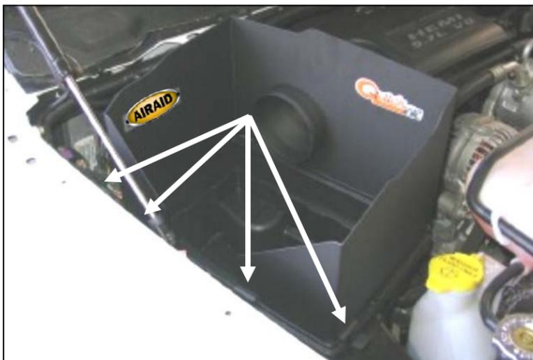
**3.** Position the Airaid Cool Air Dam (CAD) (#2) onto the factory airbox base. Relatch the factory clips onto the CAD. Apply the Airaid Foil Decal onto the Panel as shown.
