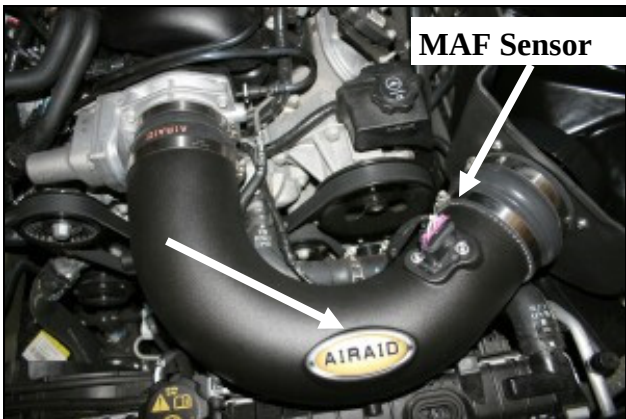
15. Install the Airaid Intake Tube (#2) into the hump hose first, and then into the reducing coupler. Adjust for fit, and tighten all four hose clamps. Next install the MAF sensor into the tube and secure it using two 8-32 x 3/8" button head screws (#20). Apply the Airaid Decal onto the Intake Tube as shown.
