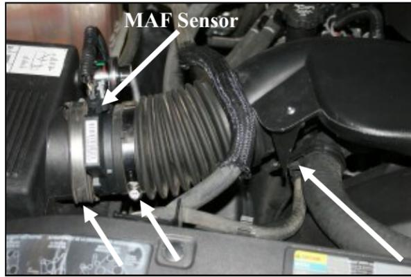
**2.** Loosen two hose clamps. One on each side of the Mass Air Flow (MAF) sensor. Using a flat blade screwdriver, disconnect the factory intake tube from the plastic clamp on the radiator hose by prying them apart.
