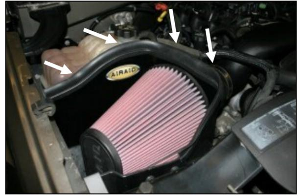
12. Install the provided weather strip (#7) along the top edge of the Airaid Cool Air Dam starting at the right fender working your way around towards the radiator. Install the Airaid Premium Filter (#1) onto the air filter adapter and tighten the hose clamp. Reinstall the factory beauty cover removed in step #1.
