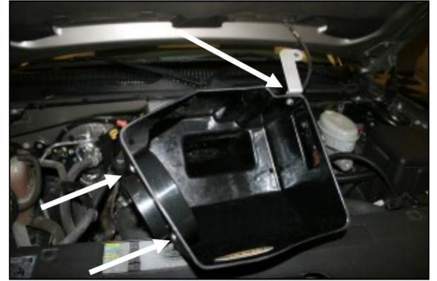
**6.** Install the filter adapter (#4) into the Cool Air Box (#3) as shown using three 1/4" Button head bolts (#8) and three 1/4" flat washers (#11). Next, fasten the bracket to the front of the CAB as shown using one 1/4-20 hex bolt (#9) two flat washers (#10), and one 1/4" Nylock nut. Refer to the drawing above for reference.
