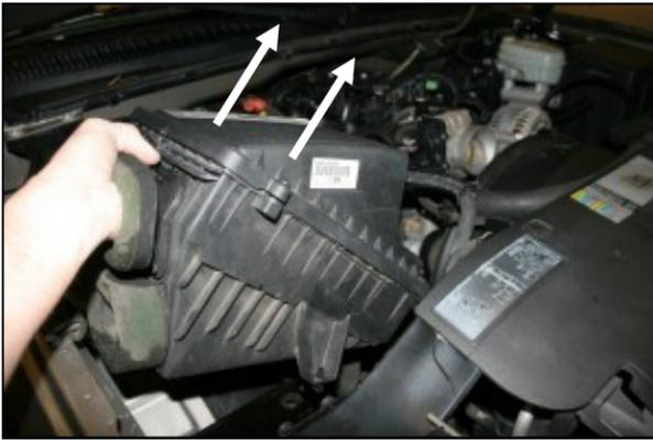
**4.** Rock the factory air box back and forth and then lift straight up remove it from the vehicle. There are only grommets holding it in, no bolts.
