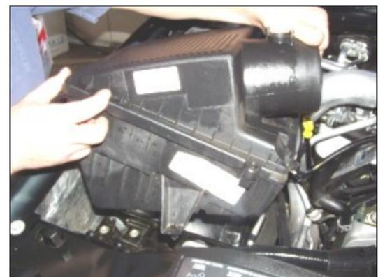
**3.** Remove the factory intake tube assembly from the engine. Rock the factory air box back and forth and remove it from its mounting. There are only grommets holding it in, no bolts.
