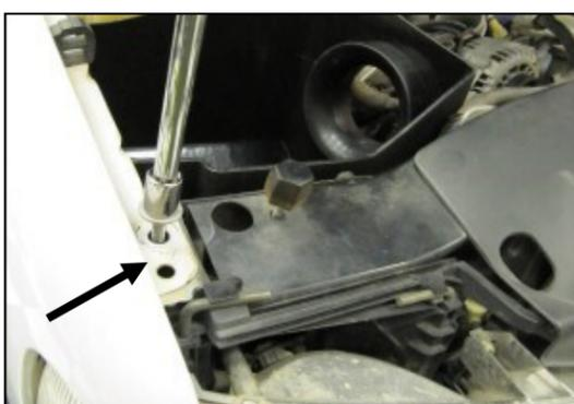
**7.** Using a 13mm socket, remove the factory fender bolt and set it aside. It will be reused in step 8.
