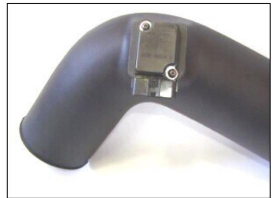
**9.** Using two 8-32 x 1/2" button head screws (#10) install the factory M.A.F. sensor in the Airaid intake tube (#2) **DO NOT USE THE FACTORY SCREWS!**
