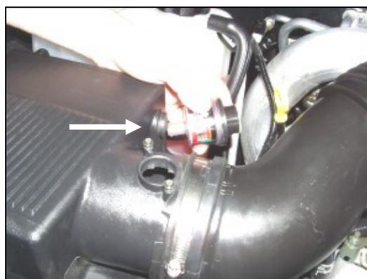
**2.** Remove the factory filter minder and grommet from the side of the factory airbox (save for reuse).
