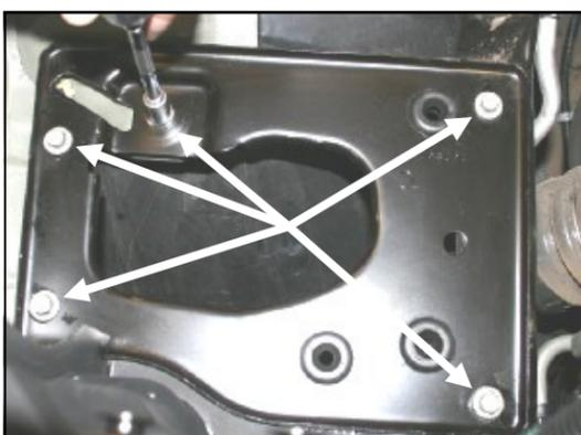
**4.** Using a 10mm socket, remove the five bolts and mounting plate from the engine compartment and set aside. Three of these bolts will be re-used in step 6.
