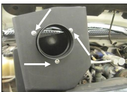
**5.** Install the Filter Adapter (#4) onto the Cold Air Box, or CAB (#3), as shown using the three 1/4-20 Button Head Bolts (#8) and 1/4" Washers (#9).
