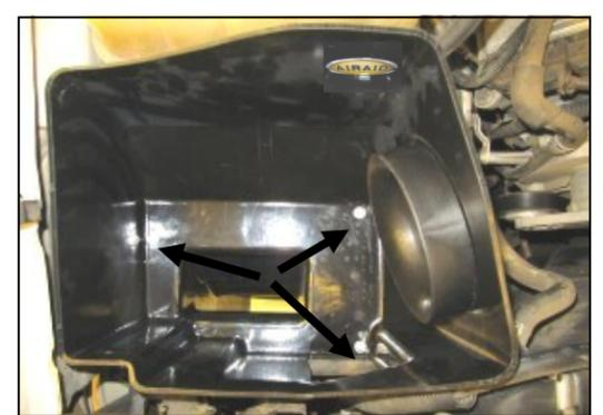
**6.** Install the Airaid CAB into the vehicle replacing the factory airbox. Secure the CAB using Three of the factory bolts from step 4. Do not over tighten Apply the Airaid Bubble Decal inside the Airbox as shown.
