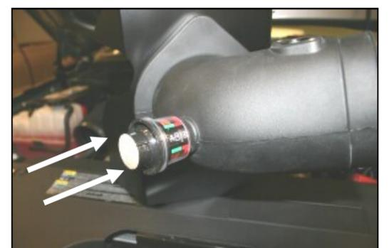
**9.** Re-install the factory grommet and filter minder removed in step #5 into the Airaid intake tube.
