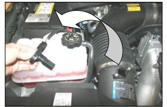
**3.** Without disconnecting the wiring harness, remove the Mass Air Flow sensor from the factory airbox, and set it aside.
