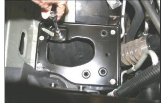
**6.** Using a 10mm socket, remove 5 bolts from the factory airbox mounting plate. Remove the plate from the vehicle.
