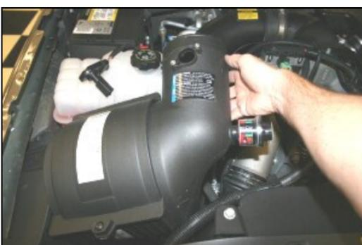
**4.** Slide the flexible intake tube off of the factory airbox and then rock the airbox back and forth to free it from the mounting grommets, next lift it straight up and remove it from the vehicle.
